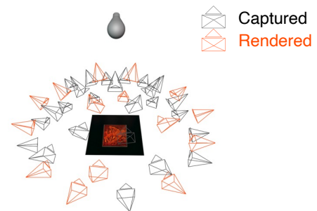
Fig. 1 Schematic of our approach: The hologram playback is captured with a sparse set of images from multiple viewpoints (black cameras). NeRF renders the novel views from new perspectives (red cameras) to provide a "seamless" viewing experience of the digitized hologram.
